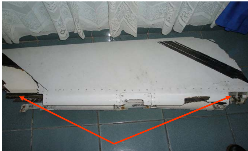
Figure A2 : Part of right elevator showing upper surface (Red arrows point to hinges). Found floating in the sea close to Sulawesi island (between Pare-pare and Baru, South Sulawesi) Makassar Strait
