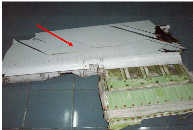
Figure A4 : Part of left elevator showing lower surface. Found floating in the sea off the coast near Pare-Pare
