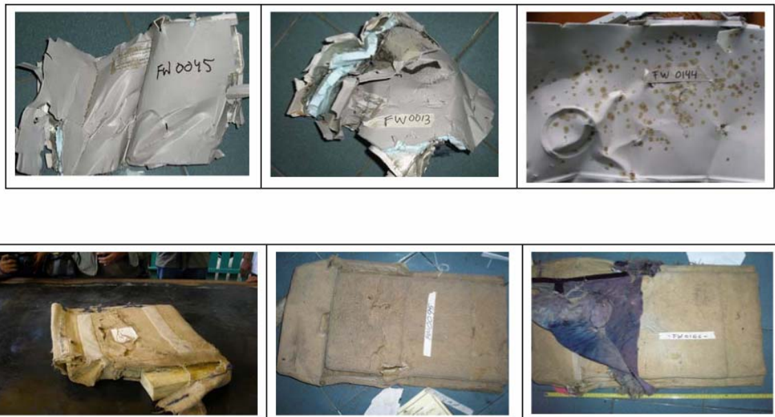
Figure A9 : Seatback tray tables (top row) and seat cushions (lower row)
