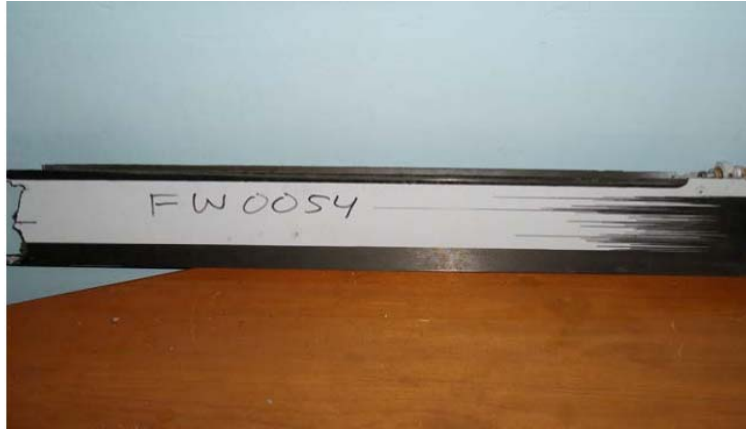
Figure A5 : Part of elevator tab. Found floating in the sea off the coast near Pare-Pare
