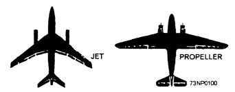
Figure 13-2.—Twin and multiengine aircraft recognition characteristics.
