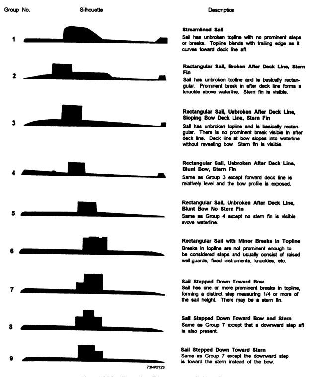
Figure 13-23.—General profile appearance of submarines.
