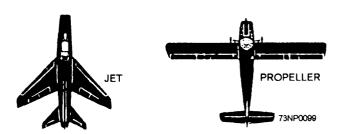
Figure 13-1.—Single-engine aircraft recognition characteristics.
