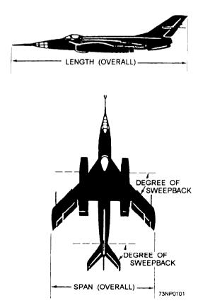
Figure 13-3.—Aircraft measurements.
