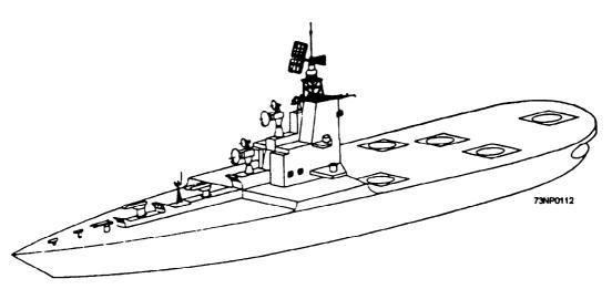
Figure 13-14.—Helicopter cruiser.
