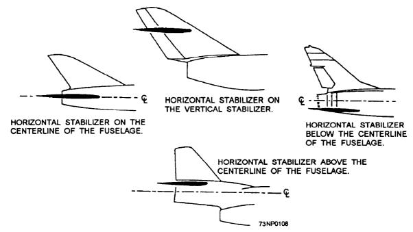
Figure 13-10.—Position of the horizontal stabilizer.
