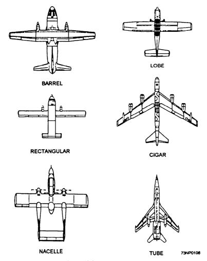
Figure 13-8.—Fuselage shapes
