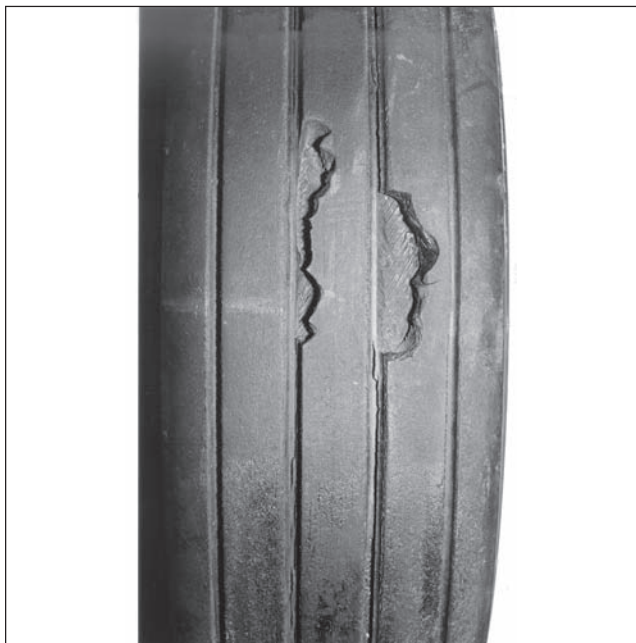
Figure 3-9. Tread Chunking and Groove Cracking
