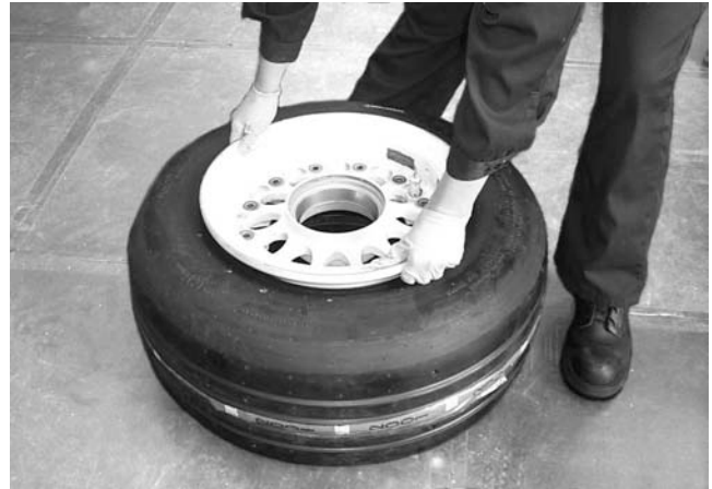
Figure 4-14. Inserting One Wheel Half into Tire
