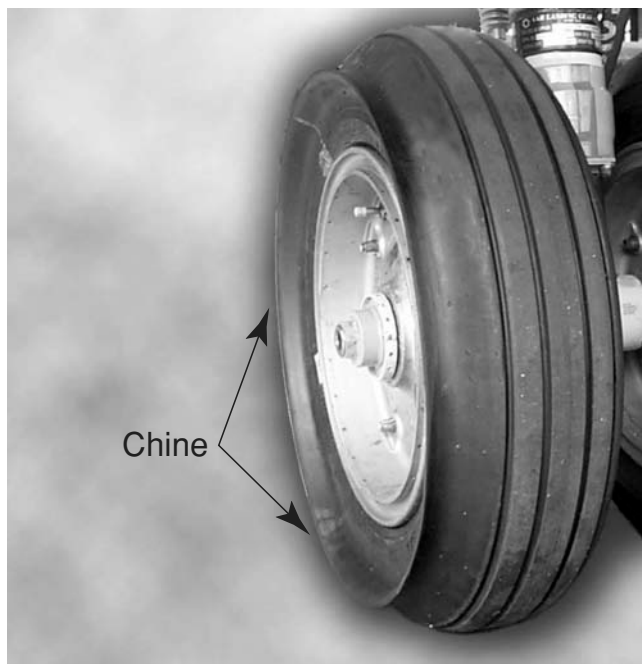
Figure 2-8. Chine Sidewall Design
