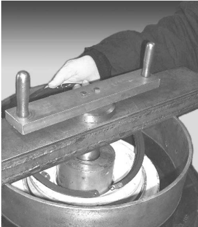
Figure 4-7. Removing Locking Ring
