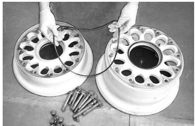
Figure 4-15. Lubricating Wheel Seat
