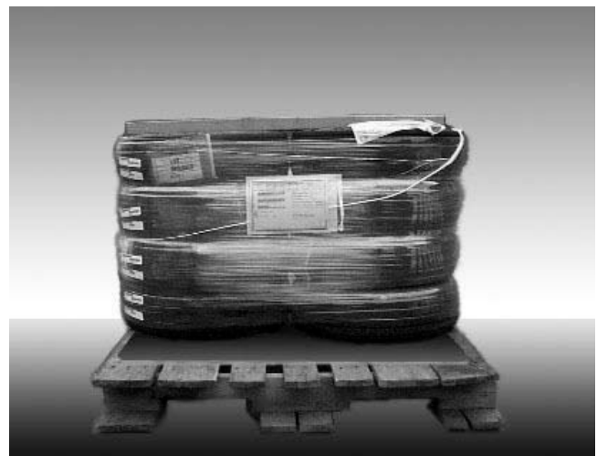
Figure 6-2. Properly Palletized Tires (Non-Assembled) for Shipment
