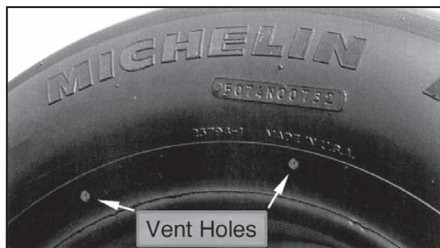
Figure 2-9. Vent Hole Markings on Sidewall
