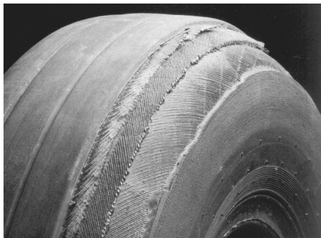
Figure 3-11. Tread Rib Peeled from Tire
