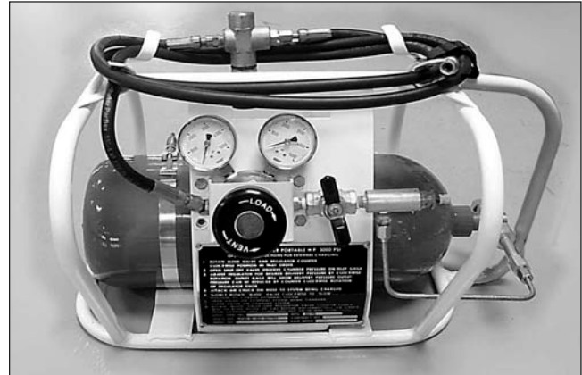
Figure 3-21. Portable High Pressure Cylinder
