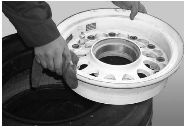
Figure 4-8. Clean Wheel with a Cloth Prior to Installation In the Tire
