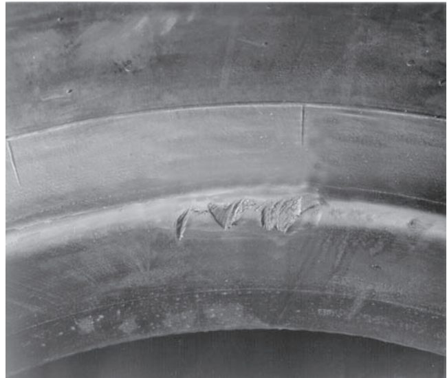
Figure 4-1. Damaged Tire Beads
