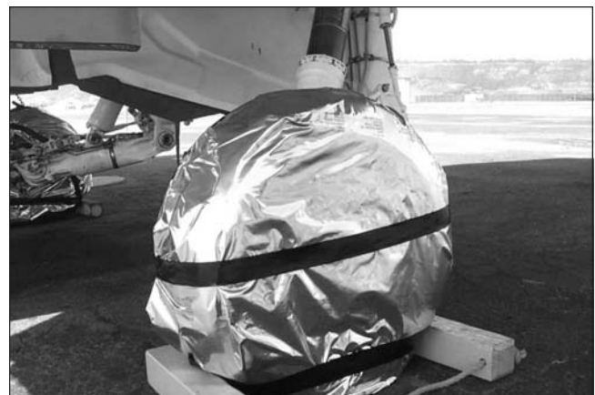
Figure 3-6. Protective Cover for Aircraft Tire
