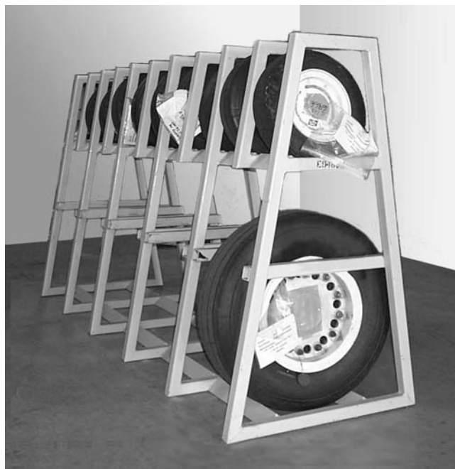
Figure 6-1. Suitable Tire Rack for Tire Shop Application (Varied Size Tires)
