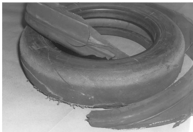
Figure 3-12. Tread Thrown From Tire Casing
