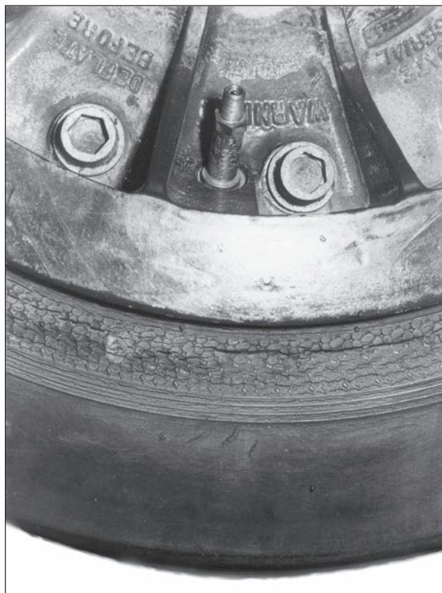
Figure 3-8. Circumferential Cracks on Tire Sidewall
