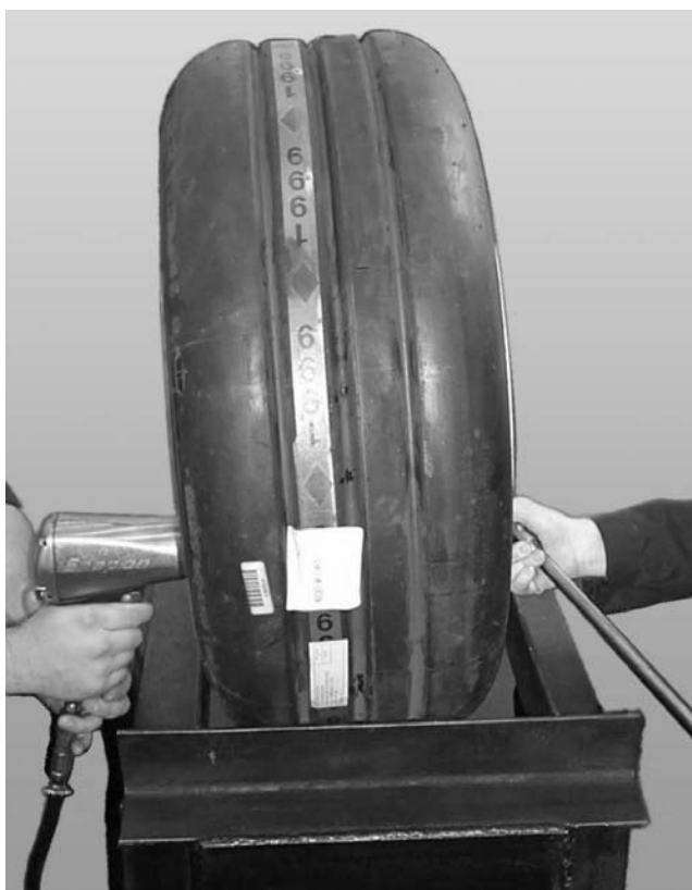
Figure 4-11. Tightening Wheel Bolts with a Pneumatic-Powered Impact Wrench
