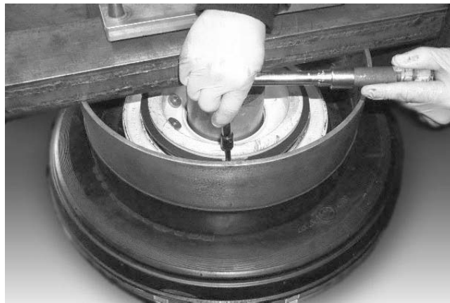
Figure 4-13. Installing the Demountable Flange
