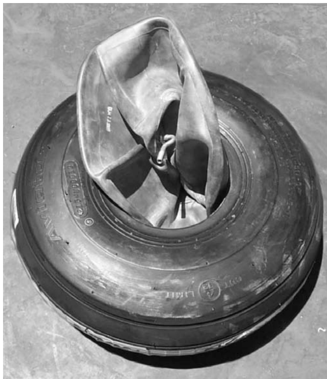
Figure 4-9. Inserting Tube in Tire
