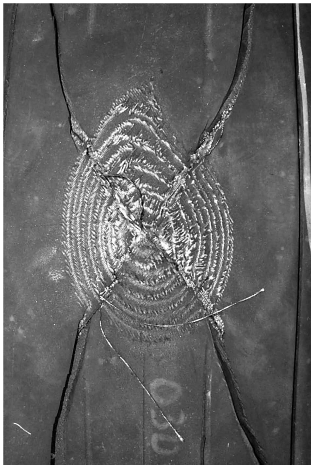
Figure 3-3. Skid Spot Caused by Severe Brake Application
