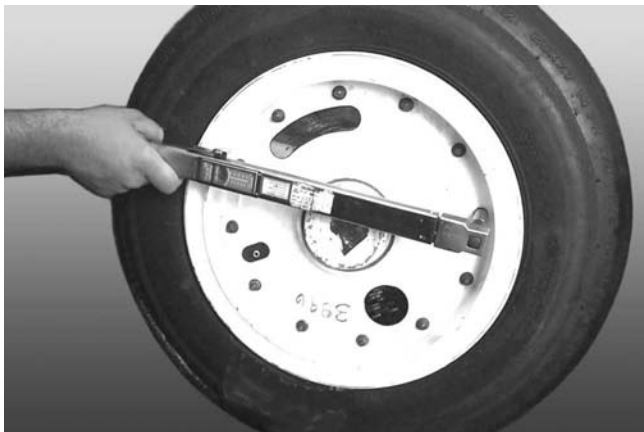
Figure 4-12. Tightening Wheel Bolts with a Torque Wrench
