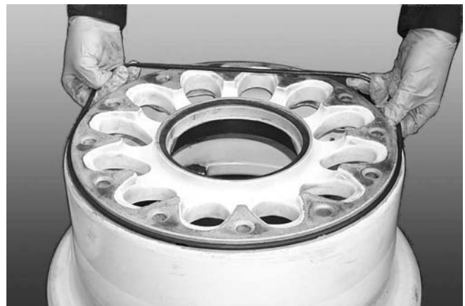
Figure 4-16. Installing Wheel Seal in Tubeless Tire Wheel
