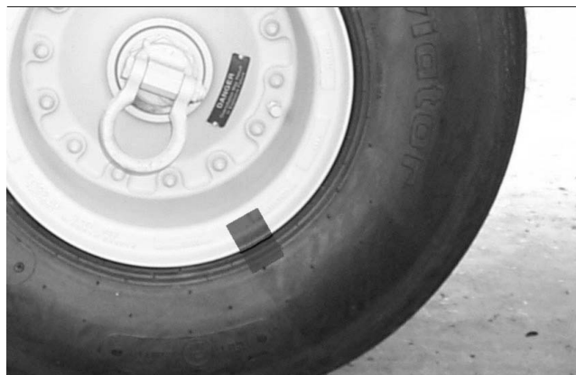
Figure 4-20. Tire Slippage Index Marking
