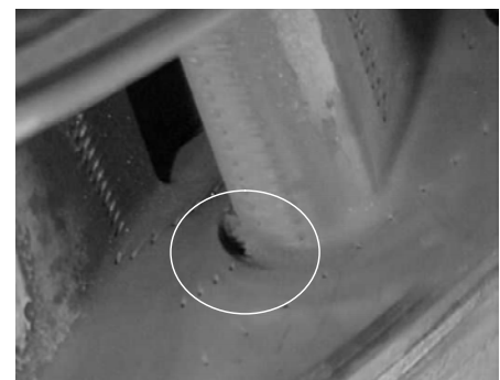
Fig. 3b. Actual hardware showing effects of the horseshoe vortex on a first vane
