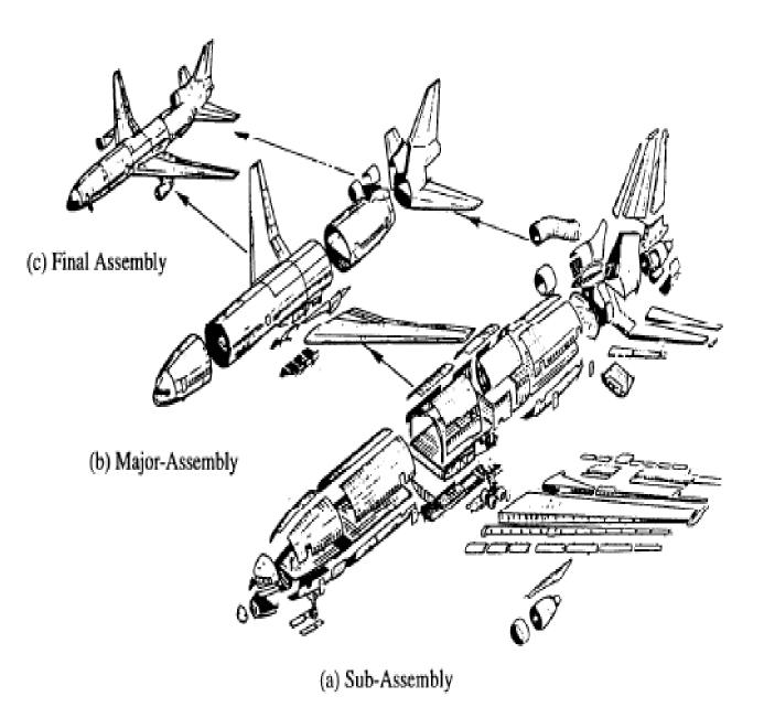
Fig. 1.4.2 Lockheed L-1011's Sub-assemblies and Final Assembly
