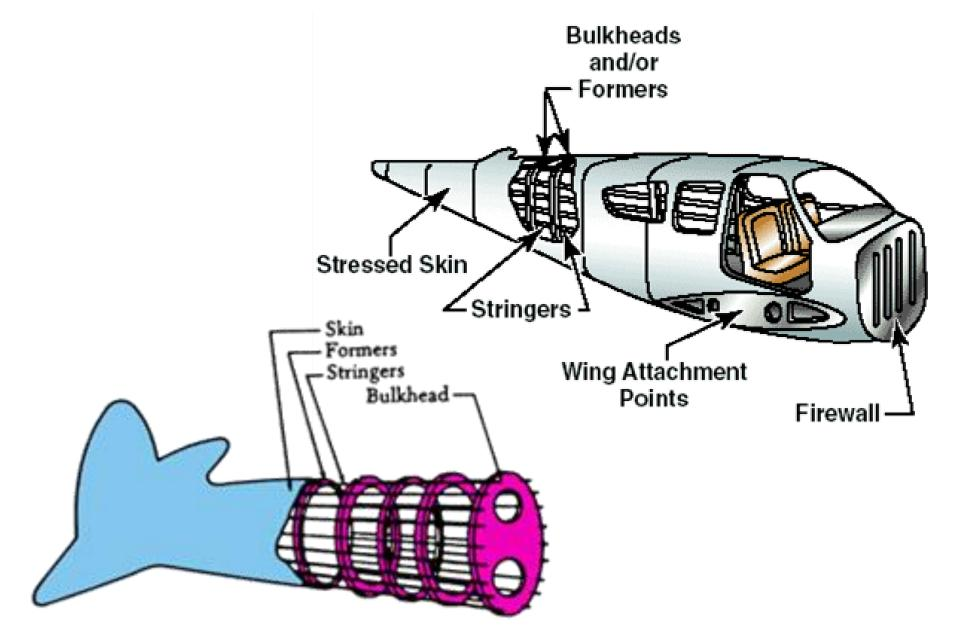
Semi-monocoque Structure of an airplane
