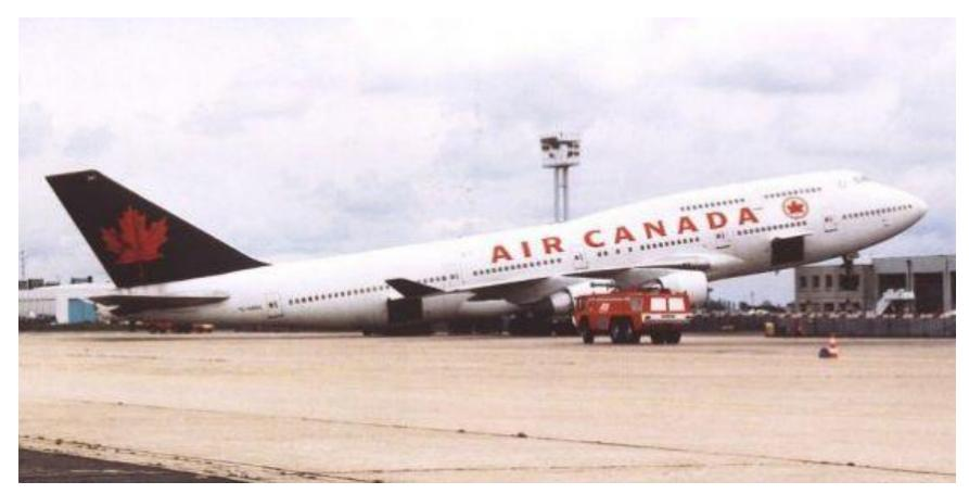
Picture from www.allstar.fiu.edu/aero/flight14.htm Improperly loaded Boeing 747
