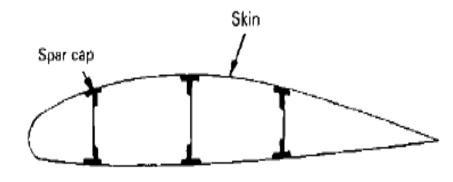
Three spar wing - all bending materials concentrated at the spar caps
