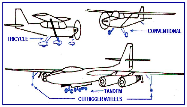
Figure 1-8 Three basic types of landing gear arrangements
