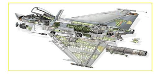
•Some items, such as wing spars, act almost entirely as one type of member, but others act as different members for different loads. For instance, the main spar near the fuselage will transmit load in bending and in shear.
