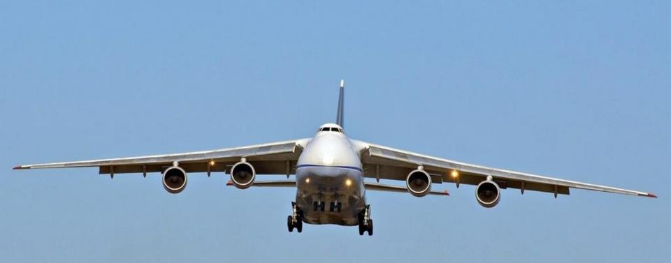
Antonov 124, USSR, 1982 Take-off mass 402 ton, payload 150 ton, wingspan 73.3 m
