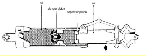
• The gas or oil will stay slightly compressed when it has the weight of the aircraft on it, so it is cushioned whilst taxying.
