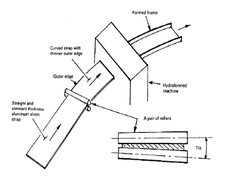
A common process of forming fuselage frame.
