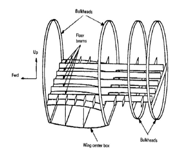
Typical transport fuselage center section floor beams arrangement.
