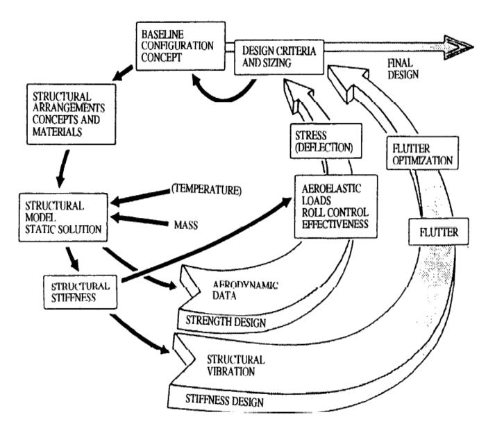
Fig. 1.1.1 Structural Analytical Design Cycles
