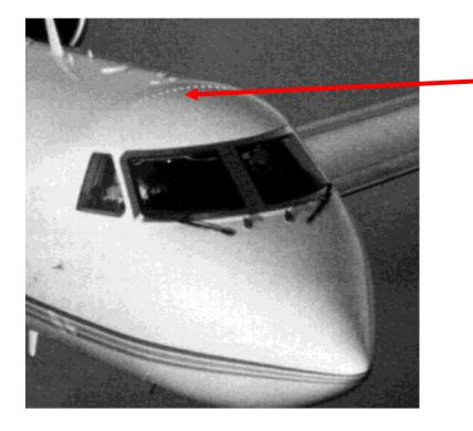
Shock wave causes flow separation in this region. Vortex generators fix problem. However, shock wave remains causing drag and considerable.
