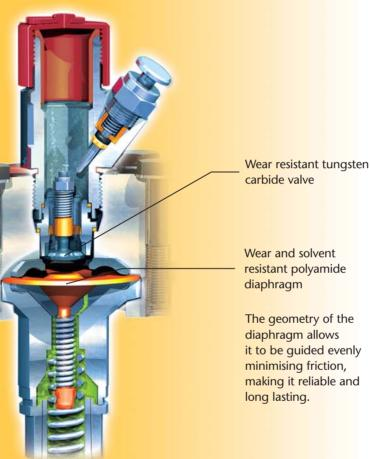
QLS technology (Quality Long Stroke technology) is the new generation of patented long stroke diaphragm equipment from Wagner.
