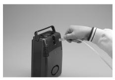
Figure 9: Connecting Cannula to FreeStyle's Oxygen Outlet
