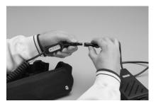
Figure 8: AirBelt Battery Charging
