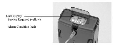
Figure 16: Indicator of Required Inspection/Service
