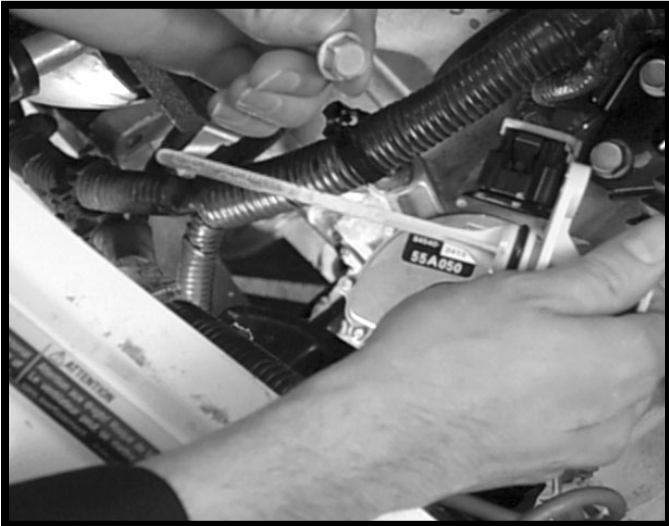
Figure 8-3, Checking the Fluid Level
