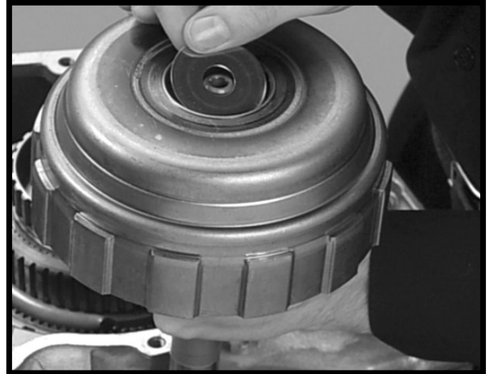
Figure 9-6, Replacing the Selective Thrust Washer
