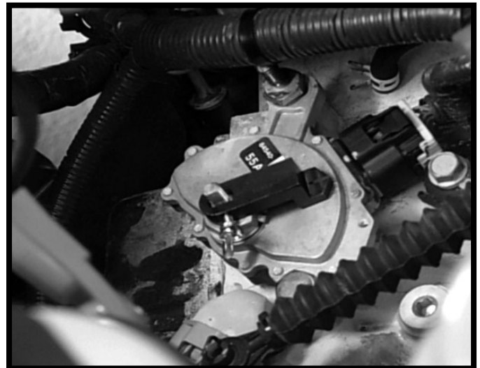
Figure 8-2, Park/Neutral Position Switch Adjustment
