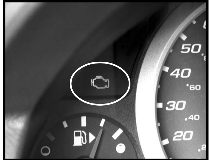
Figure 6-3, In Emergency Mode, the MIL Will Illuminate
