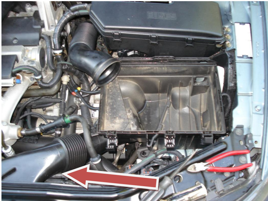
Remove the airbox lid. Then remove the ducting to the front of the radiator support from the airbox.
