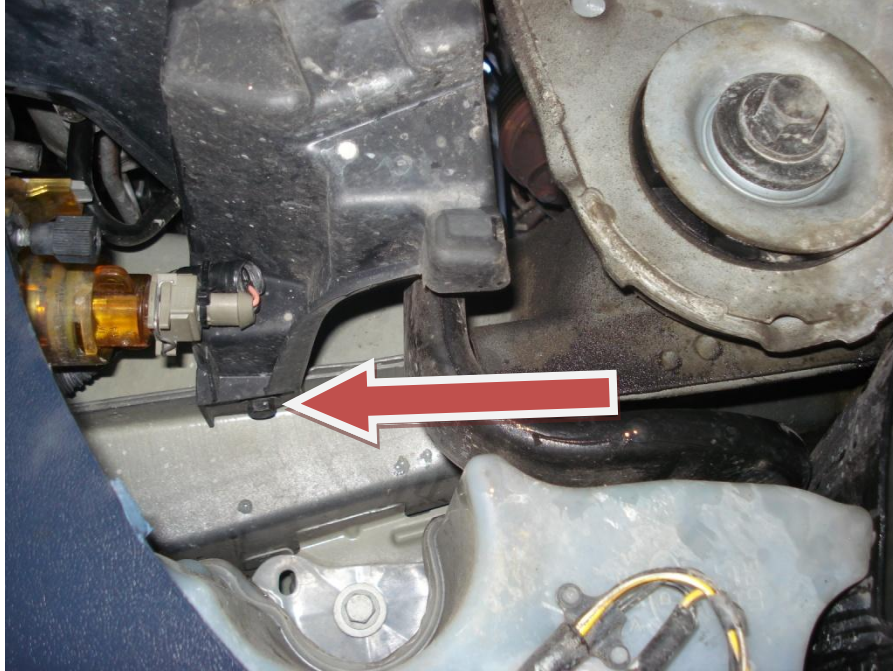
10MM bolt location. Passenger side shown.
