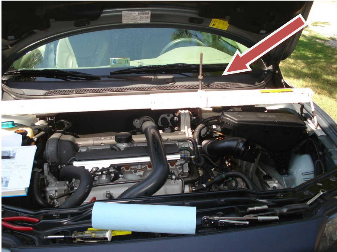
The lift is the white bar across the engine bay. The threaded rod hooks into the lift bracket on the engine.
