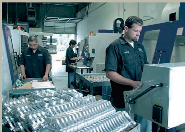
Three Silray Akira Seiki mills (a V4 Performa, an SV1000 and an SV1300) are grouped into a work cell. Operators are (foreground, right) CNC machinist Billy Roncallo, CNC machinist Mario Rosa (left front) and CNC machinist programmer Quoc Ta (background).
