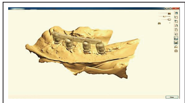
Fig. (8) Superimposed round bar virtual pattern on the four virtual abutments.
