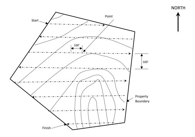
FIGURE 3. Systematic Application of Point Frequency Method.
