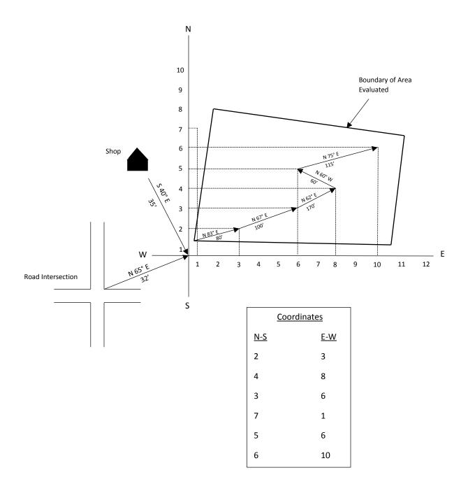
FIGURE 1. Locating Points for Point-Frequency Method.
