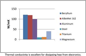
Using beryllium materials in heat sink cores has improved life of some electronic modules as much as 8 times.
