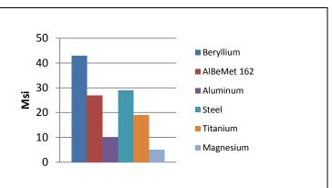
Modulus (stiffness) of material being almost same as steel. In stiffness driven apps, AlBeMet<sup>®</sup> can provide 50% weight savings.
