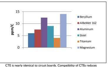
thermal strains between cores & circuit boards. Compatibility of CTEs reduces thermal strains between cores & circuitry components resulting in fewer failures. In an application the CTE of the base material is a dominant contribution to thermal mechanical stress.
