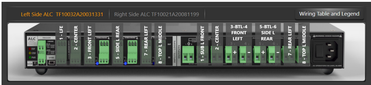
AUTOMATOR™ WIRING GUIDE SHOWING OUTPUTS 3-4 AND 5-6 BRIDGED
