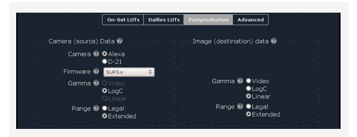
For compositing with computer generated elements images are normally converted to a linear encoding. The web application at <u>www.arridigital.com</u> offers LUTs for this purpose as well.
