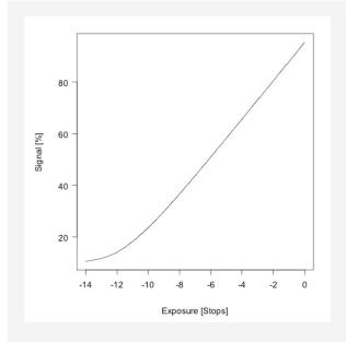
Figure 1: Log C curve used in ALEXA SUP 3.x Note also that the curve does not start at a signal level of zero. This is mostly done to be compatible with scanned negative where the clear base, which is black in the image, is traditionally represented by a code value around 95 in the 10 bit encoding (that is a signal level of approximately 10%).
