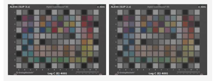
Open this  $\underline{\text{HTML}}$  file in your browser to see a demonstration of the differences in Log C between SUP 2.x and SUP 3.0. Notice the difference in color saturation between the image from SUP 3.0 on the left side and the image from SUP 2.x on the right side.
