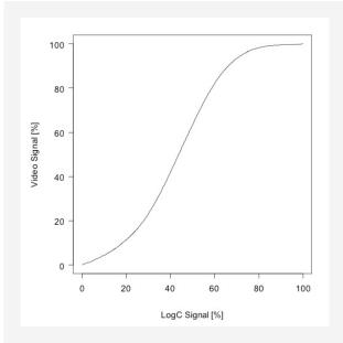
Figure 2: Tone-map curve (including video gamma correction)
