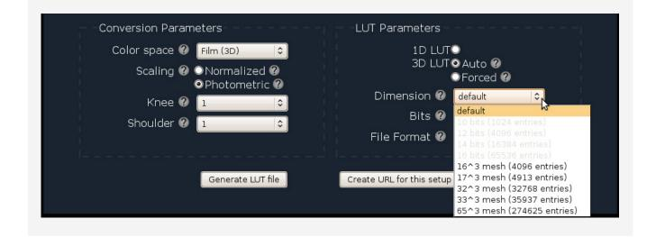
The bit size of a one-dimensional LUT rules how many distinct input values can be encoded. The preset for all LUT formats uses a sensible default for those formats that support multiple sizes. For special needs, you can change this size. Some formats are only available in a fixed size and they will ignore this setting.
