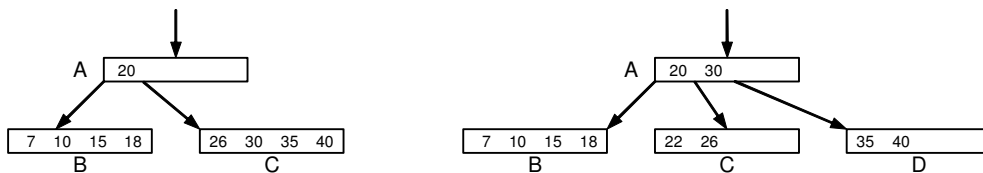
Fig. 4.44. Insertion of key 22 in B-tree
