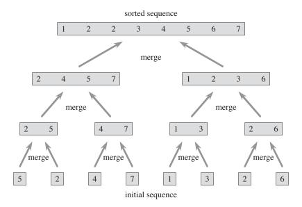
**Figure 2.4** The operation of merge sort on the array A = (5, 2, 4, 7, 1, 3, 2, 6). The lengths of the sorted sequences being merged increase as the algorithm progresses from bottom to top.
