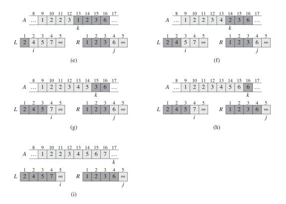
**Figure 2.3, continued** (i) The arrays and indices at termination. At this point, the subarray in A[9..16] is sorted, and the two sentinels in L and R are the only two elements in these arrays that have not been copied into A.
