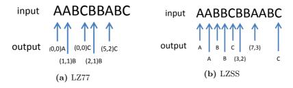
Figure 3.1: Output example of the original LZ77 versus LZSS. Notice, that on LZ77 every output is a reference pointer with either a length = 0 and the current character, or length > 0 and the next character. The output for LZSS is with a minimum matching length of 2
