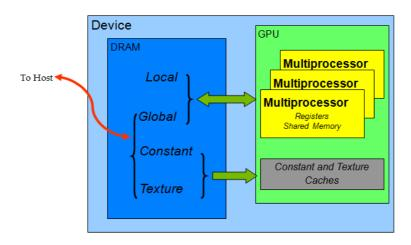
Figure 4.2: An illustration of the memory spaces on a CUDA device  $^2$
