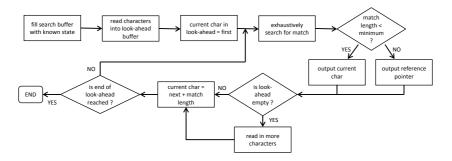
Figure 3.3: State diagram over the LZSS compression process
