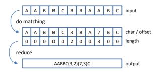
Figure 5.2: An illustration of the two-dimensional output form of the CULZSS, that afterwards needs to be stripped of the redundant data to produce the correct form of encoded information
