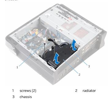
Lift the radiator and hold it as shown in the image below to remove the thumbscrews that secure the processor cooler to the system board.
