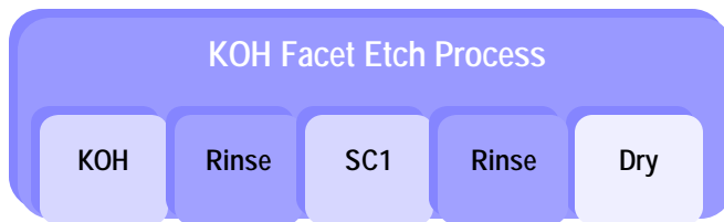
Figure 5. Example of a KOH facet etching configuration for a wet bench.
