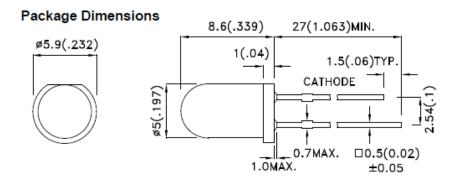
As you can see, the main diameter of the LED is 5mm (its a '5mm LED') and there's a lip that makes it around 6mm. The lip can make it handy if you're gluing the LED into a drilled hole, so it doesnt fall through. The datasheet also tells you which pin is the cathode and other lengths and sizes. Note that the figures are in mm with the inches in ()'s afterwards.
