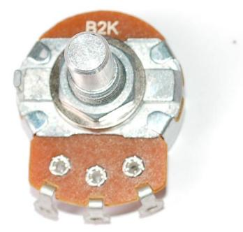
Potentiometers, like resistors, have an Ohm value. For example, this potetiometer is a 2Kohm (its printed up top). Potentiometers have three pins, two 'outer' and one 'middle' pin. The middle pin is sometimes called the wiper.
