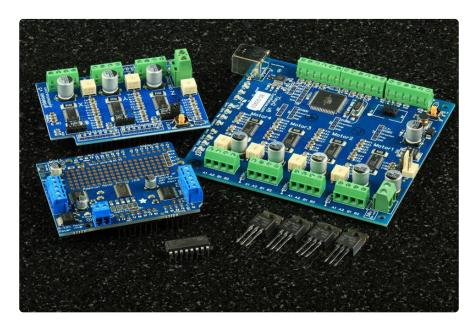
Driving a stepper motor is a bit more complicated than driving a regular brushed DC motor. Stepper motors require a stepper controller to energize the phases in a timely sequence to make the motor turn.
