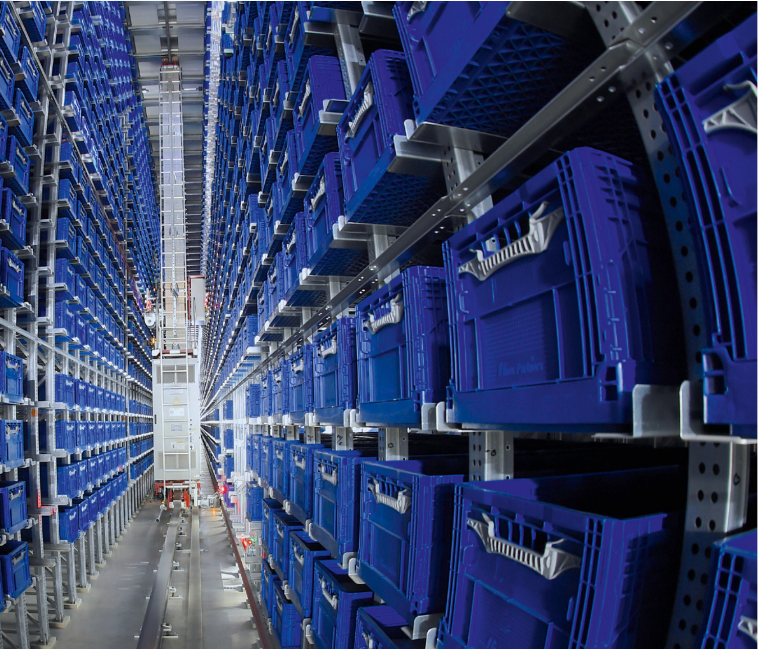
Highly dynamic stacker cranes ensure a permanent optimization of the goods distribution in all warehouse aisles.
