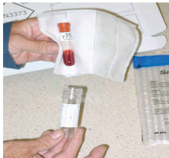
Figure 129: Wrap the sample in absorbent material and place in a leak proof plastic container.
