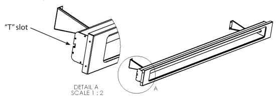
Adjustable wall/ceiling brackets are furnished with all SL series heaters. Brackets have positive stops at 30° & 60°. When used, they allow heater to be fastened to wall and then tipped down to 60°. For ceiling mount tilted to 30° max. Brackets are positioned along a "T" slot on back of unit. You must maintain a minimum distance between to ensure a stable installation.
