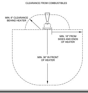
NOTE: <u>DO NOT</u> mount the heater on a vertical axis. Such installation will reduce the life of the element and will automatically void the product's warranty. Heater must be installed with the quartz tube horizontally level. For maximum tube life, use a "carpenters level tool" to find the optimum level position for the heaters' body.
