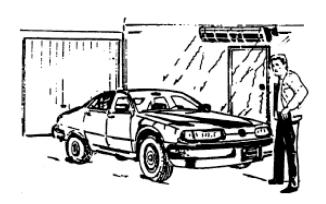
Install fixture to heat the area from the "cold side" if possible. This helps compensate for increased body heat losses due to exposure.
