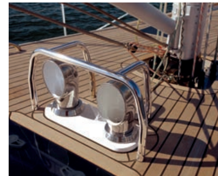
Stainless steel ventilation dorades are mounted on the coach roof, with stainless steel protection bar, provide excellent ventilation into the accommodation.
