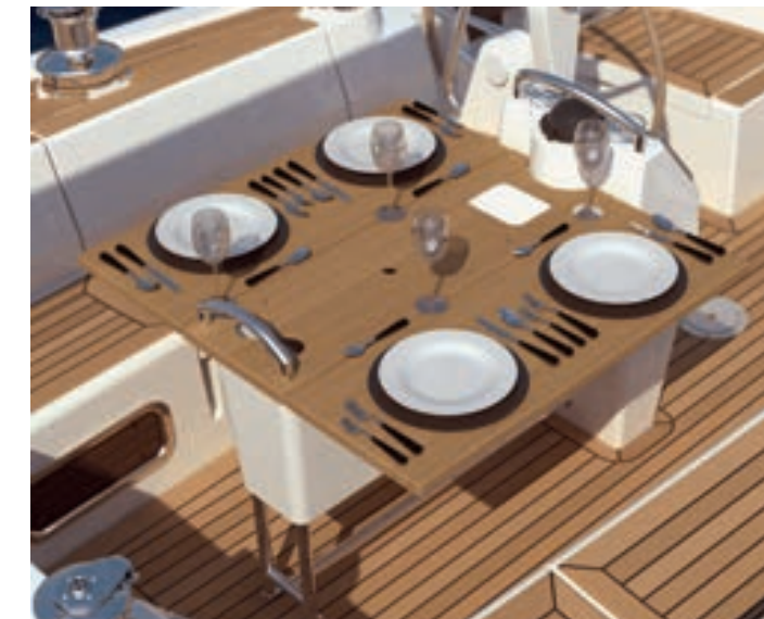
Folding teak cockpit table with GRP instrument support designed to fit a chart plotter and binnacle compass. Storage in centre of table.
