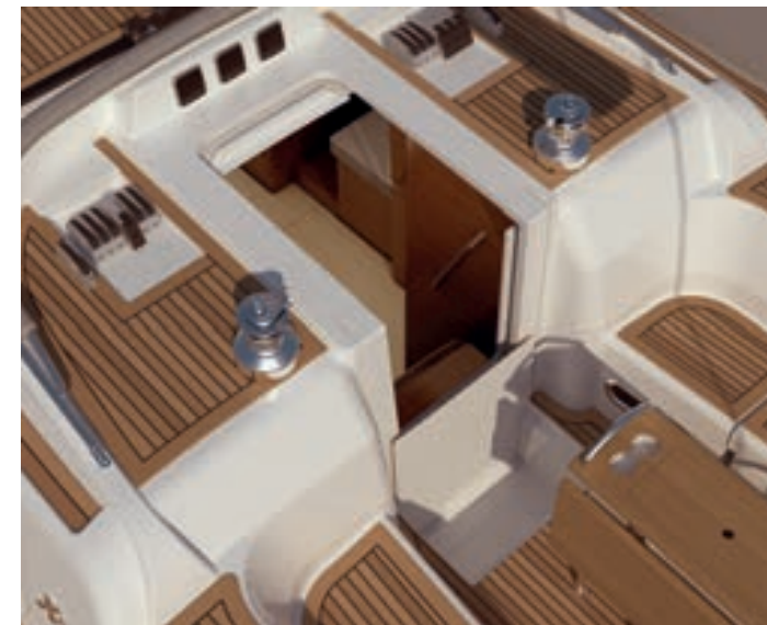
All halyards pass below the deck surface and are stored in the cockpit floor self draining "bin". Self-draining, acrylic dropboard is supported by gas struts for easy adjustment.
