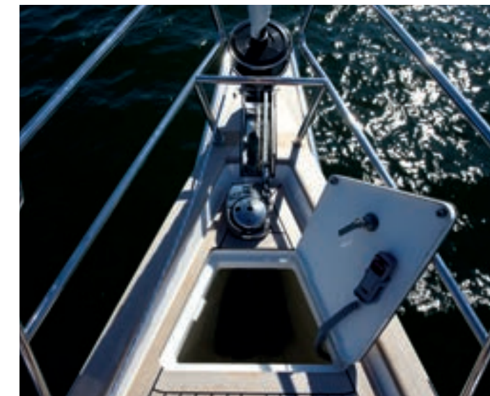
The foredeck locker, with integrated self-draining anchor chain compartment. The electrical anchor winch can be fitted with a capstan version to operate mooring line.
