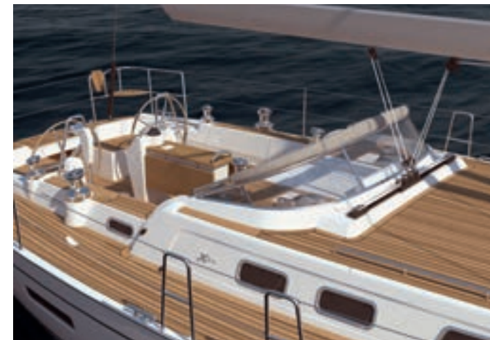
Xc 42 comes optional with an aluminium framed windshield with toughened glass.
