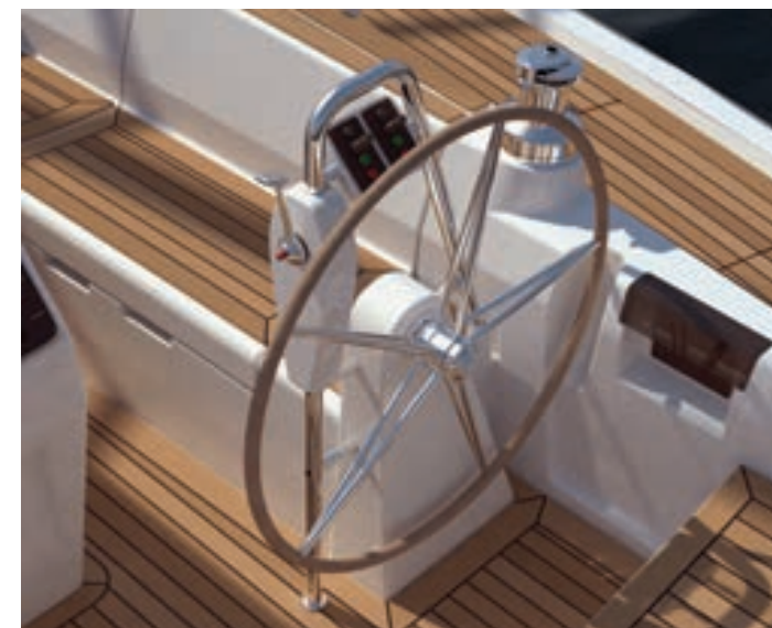
The 'standard' Xc 42 comes with stainless steel wheel crash bars. Optional enlarged crash bars with integrated engine throttle and/or
