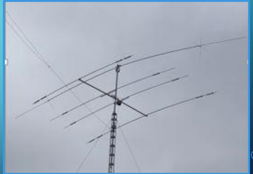
Tribander: Mosely TA-53 Five-band Antenna (bottom antenna) Rotary Dipole: Trapped 40m dipole (top antenna)
