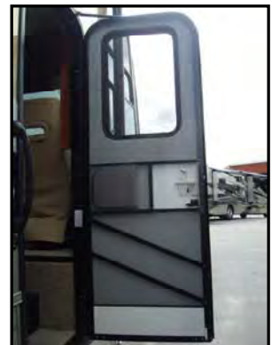
Figure 13-6. Front Door & Screen Door
