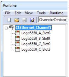
Each device appears under a single channel, called "CLEthernet\_ Channel1". In this configuration, the driver moves from one device to the next as quickly as possible to gather information at an effective rate. As more devices are added or more information is requested from a single device, the overall update rate begins to suffer.
