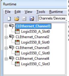
Each device has now been defined under its own channel. In this new configuration, a single path of execution is dedicated to the task of gathering data from each device. If the application has fewer devices, it can be optimized as shown here.
