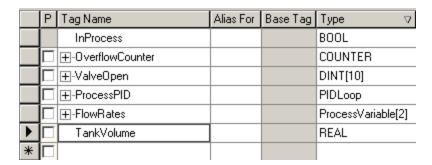
2. After performing Automatic Tag Database Generation from this controller, the server produces the following project.
