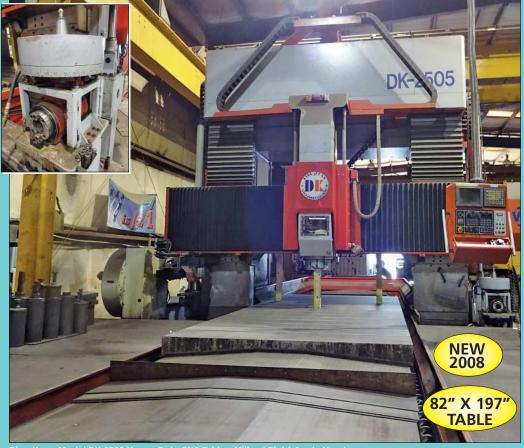
Ding Koan Model DK-2506 Heavy Duty CNC Bridge Mill w/ Right Angle Head
