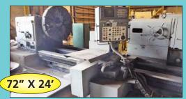
72" x 24' (Approx.) Niles Zerbst Heavy Duty Flat Bed CNC Engine Lathe
