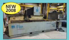
Flow Model IFB CNC Water Jet Cutting Table
