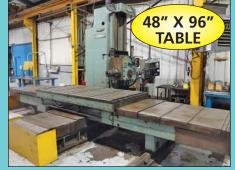
4" Nomura / Olympia Model B-100WB Four-Axis Table Type CNC Horizontal Boring Mill
