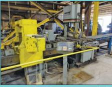
21" x 22" Marvel Model MV525PC/1 Automatic Tilt Frame Vertical Band Saw
