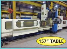
Kao-Ming Model KMC-4000SD CNC Bridge Mill
