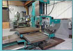
4" Shibaura Model BT10B-R1 Rotary Table Horizontal Boring Mill
