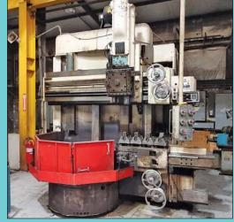
48" Bullard Model Cutmaster Vertical Turret Lathe
