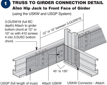
Attach to USW18 w/3 -#10 screws (3.5USGP) to USGP w/4 -#10 screws
