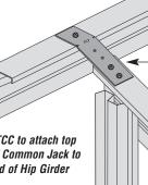
Attach USTCC to top chord of Hip Girder with (1) #8 or #10 low profile SDS. Bend to the required angle and attach to Common Jack with (2) #8 or #10 low profile SDS.
