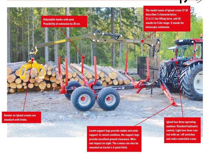
The IGLAND Swingtrac System is a uniquely composed product, which makes it easier to maneuver in tough terrains, where logs and rocks can be a barrier to a timber trailer. The Swingtrac system makes it possible to creep through the terrain, using a powerful push effect (4 ton), which comes from locking the rear wheels on the trailer, combined with the hydraulic steering on the bogie.
