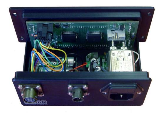
Install a shorting jumper across pins 3 and 4 of the gray connector on the rear of the main pc board to prevent the head type from being changed.
