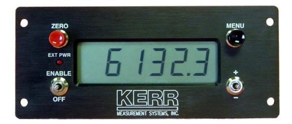
The Backup Depth System is designed to be an independent depth measurement indicator for mounting inside a wireline unit. The depth is measured by a magnetic pickup mounted in the measuring head and displayed in either feet or meters at the display unit. The unit is powered by three internal batteries. It can be connected to an external AC or DC power source to keep the batteries charged.
