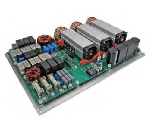
Figure 4: MSCSICPFC/REF5 is a three-phase Vienna PFC reference design. (Image: Microchip Technology)
