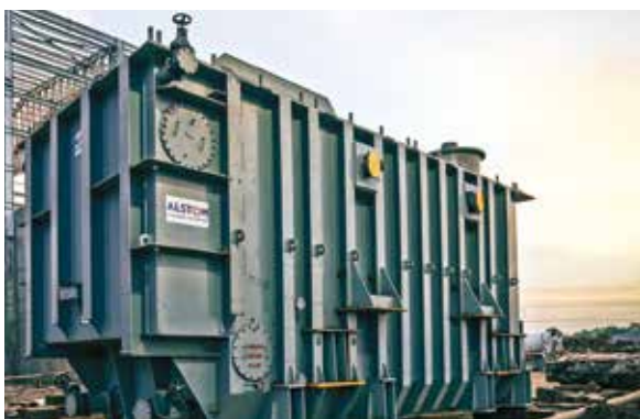
Despatch of India's First 'Make in India' 800kV UHVDC transformer for PGCIL Champa Kurukshetra site
