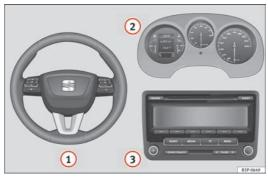
Fig. 1 Display and handling components of the Bluetooth system.
