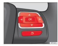
Fig. 3 Right-side buttons on the multifunction steering wheel.
