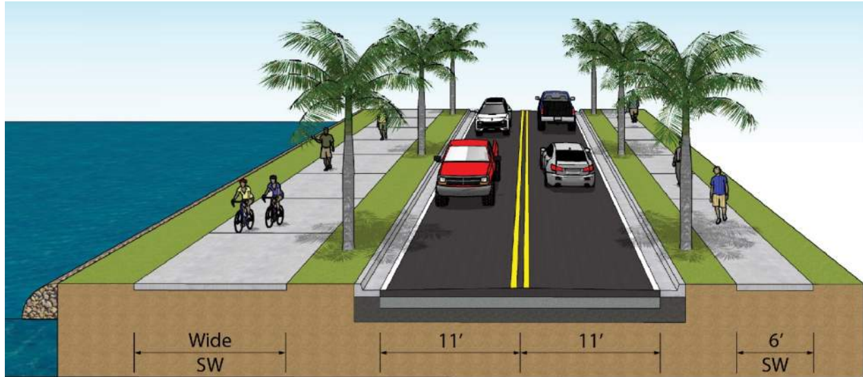
Figure 3.7 Proposed Typical Section from Sunset Point Road to Union Street
