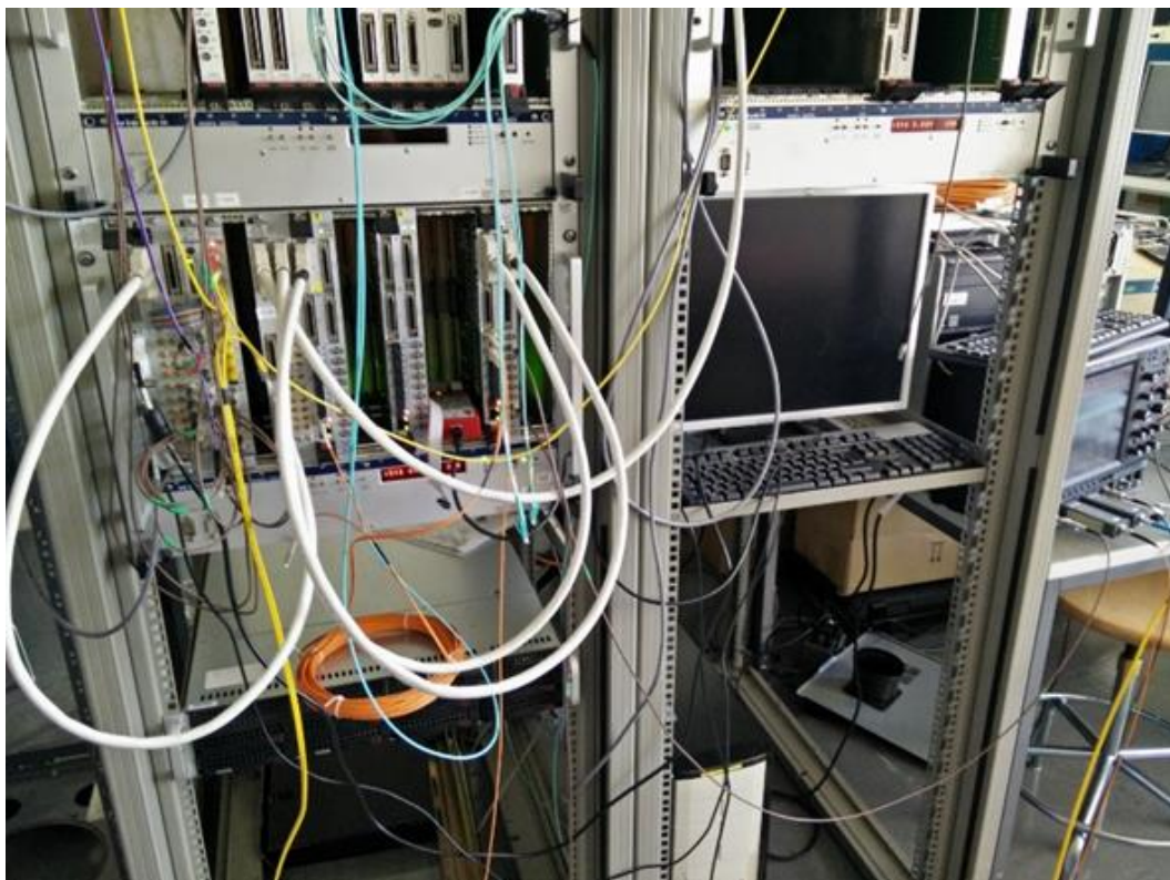
Figure 6.1.1. Typical laboratory test setup with multiple ALTI and legacy TTC modules in the same VME crate.
