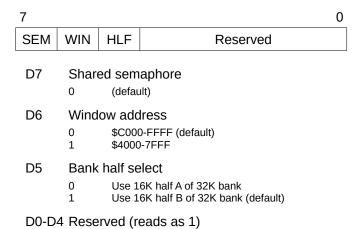
The 65C816 controls its portion of the Veronica hardware by a single register, mirrored at \$0200-020F. This register exposes the shared semaphore bit as well as banking window selection and bank half selection. Its value is reset to \$3F on power-up or soft reset.
