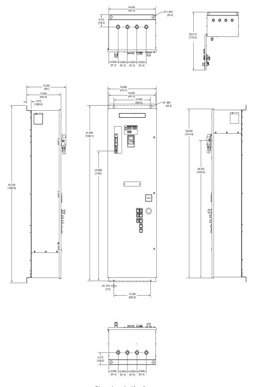
Figure 7: Size D Enclosure, Floor Mount, Type 1 and 12, 20 inches wide, 8639 Power Circuit S (Shunt Trip) only: 60–100 hp @ 208 V, 75–125 hp @ 230 V, 150–250 hp @ 480 V, and 200–300 hp @ 575 V
