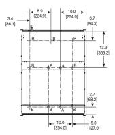
Figure 9: Size D Enclosure, Floor Mount, Type 1 and 12, 30 inches wide, 8639 Power Circuit N (Isolation Contactor) or R (Reversing): 60–100 hp @ 208 V, 75–125 hp @ 230 V, 150–250 hp @ 480 V, and 200–300 hp @ 575 V
