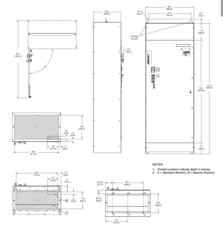
Figure 12: Size E Enclosure Outline, Floor Mount, Type 3R, 55 in. wide, 8638 and 8339 Power Circuit R (Reversing): 125–200 hp @ 208 V, 150–250 hp @ 230 V, 300–500 hp @ 480 V, and 350–600 hp @ 575 V
