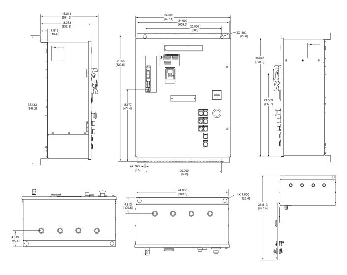
Figure 5: Size B Enclosure, Wall Mount, Type 1, 12, and 3R: 15–30 hp @ 208 V, 20–40 hp @ 230 V, 40–75 hp @ 480 V, and 50–100 hp @ 575 V
