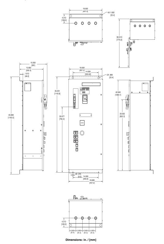
Figure 6: Size C Enclosure, Wall Mount, Type 1, 12, and 3R: 40–50 hp @ 208 V, 50–60 hp @ 230 V, 100–125 hp @ 480 V, and 125–150 hp @ 575 V
