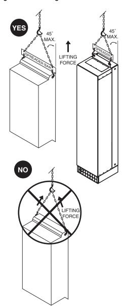
Handle the Enclosed 48 carefully to avoid damage to the internal components, frame, or exterior. When handling the controller, balance it carefully to keep it from tipping. After removing the packaging materials, the controller requires some type of mechanical lifting.
