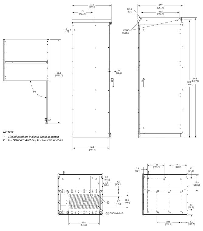
Figure 11: Size E Enclosure, Floor Mount, Type 1 and 12, 35 inches wide, 8638 and 8639 Power Circuit N (Isolation Contactor) or S (Shunt Trip): 125–200 hp @ 208 V, 150–250 hp @ 230 V, 300–500 hp @ 480 V, and 350–600 hp @ 575 V
