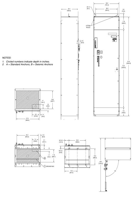
Figure 10: Size D Enclosure, Floor Mount, Type 3R, 30 inches wide, 8639 Power Circuit N (Isolation Contactor) or R (Reversing): 60–100 hp @ 208 V, 75–125 hp @ 230 V, 150–250 hp @ 480 V, and 200–300 hp @ 575 V
