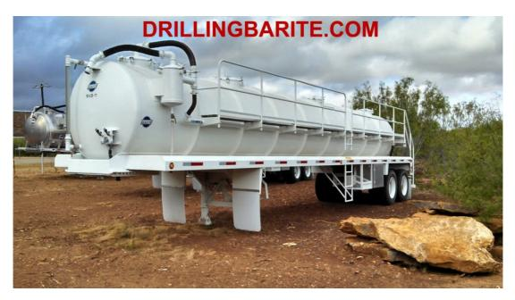
**Basic Unit** Cylindrical vacuum tank trailer non code manufactured in carbon steel A-36 with 1/4" body thickness, 1/4" bulkhead and (8) external rolled rings, . For unspecified Oilfield fluids.
