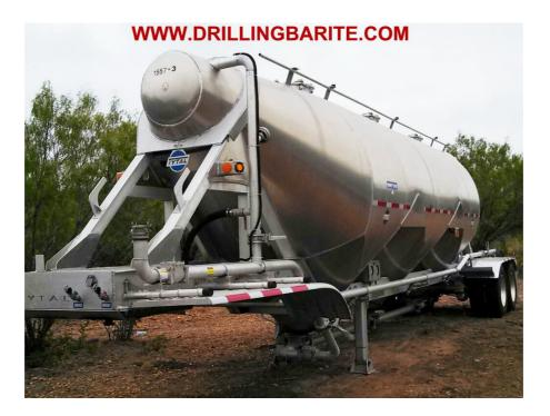
**Basic Unit** Hopper's body in aluminum 5454-H32 caliber 3/16" with diagonal reinforcements of PTR 4X4 in both endpoints and three inferiors cones of 1/4" (thickness), to transport low density solids.
