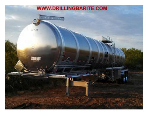
**Basic Unit** Cylindrical tank manufactured with high resistance quality aluminum 5454-H32 with 1/4" body thickness. For crude oil transportation
