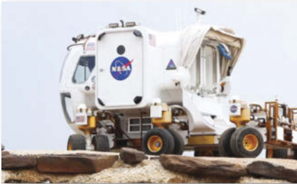
This rover includes about 70 FDM parts, including housings, vents and fixtures.
