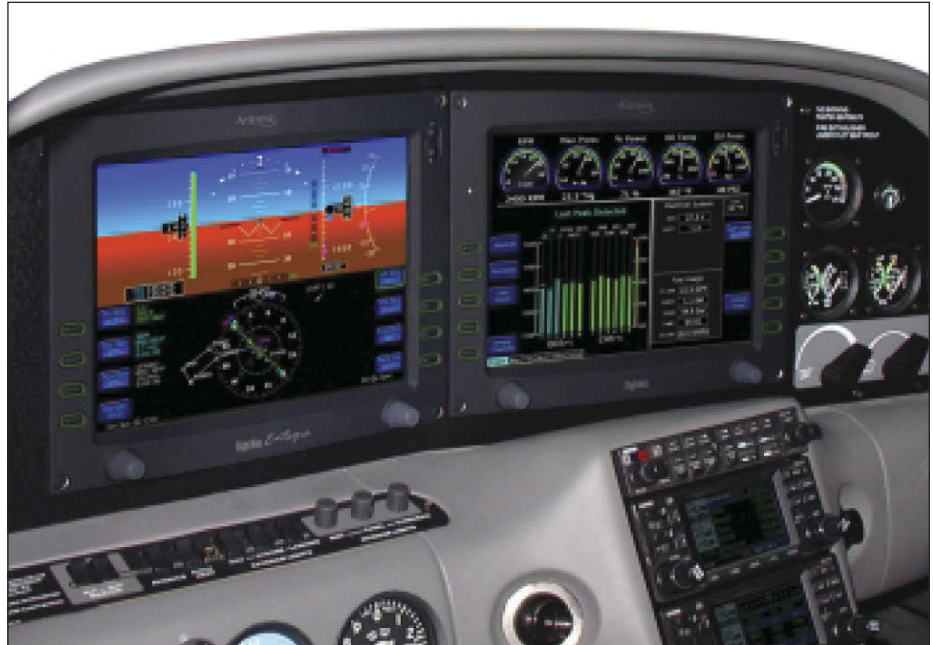
An example of a glass cockpit. In most modern commercial airplanes, including the A380, A350, and 787, the traditional “widget-based” (or WIMP) approach is mostly used for interactive cockpit displays.
