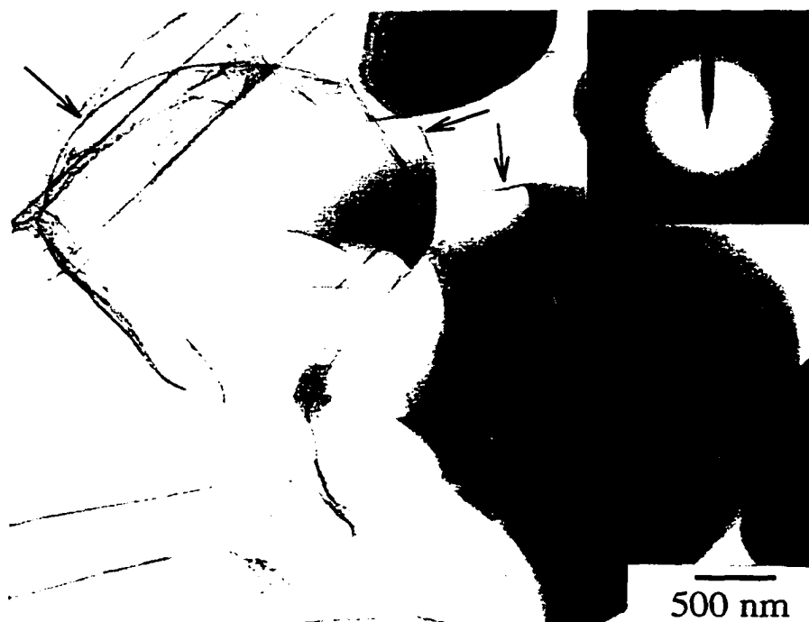
Figure 4.24. TEM micrograph and SAD pattern of the oxide film on GARS aluminum powder. The arrows indicate oxide thickness measurements.
