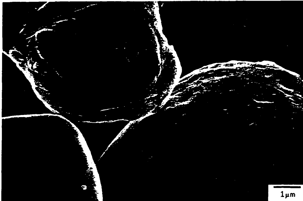
Figure 4.48. SEM micrograph of the CAA aluminum powder air sintered at 300°C for 24 hours.
