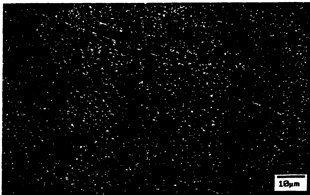
Figure 4.54. SEM micrograph showing the CIP-VCD-HIP microstructure of the GARS aluminum powder. No residual porosity is observed in the sample.
