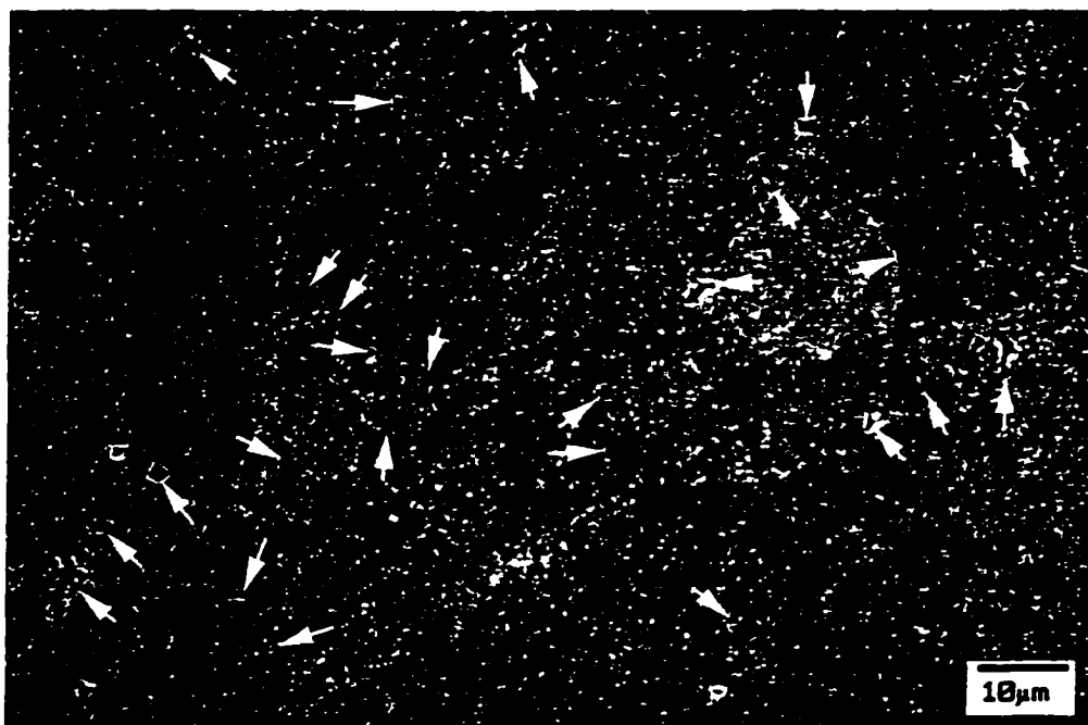
Figure 4.55. SEM micrograph showing the CIP-VHD-HIP microstructure of GARS aluminum powder. The white arrows indicate the residual porosity in the sample.
