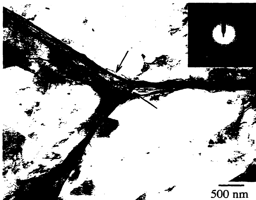
Figure 4.23. TEM micrograph and SAD pattern of the oxide film on CAA aluminum powder. The arrows indicate the oxide thickness measurements.
