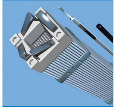
Fuel assembly, fuel rod, cladding, fuel pellet
