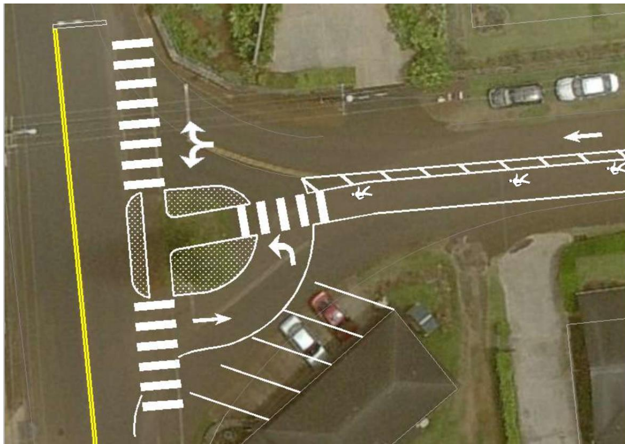
Figure 12. Sample of Low Cost Repainting Solution to Improve Pedestrian Access.
