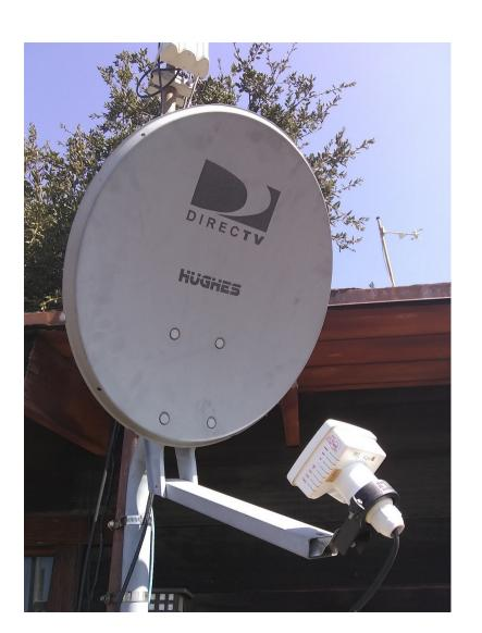
Mikrotik LDF 5 (5 GHz) installed at surplus satellite dish feedpoint using universal mount (\$8 from Amazon)
