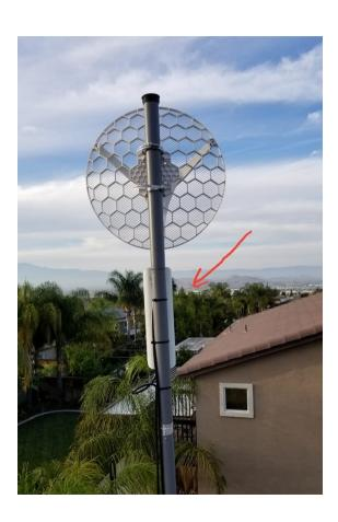
High-gain dish for access to distant network backbone node; Lower-gain node for local user access (neighborhood)
