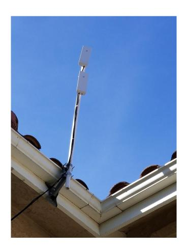
AREDN nodes for both 2 and 5 GHz; provides redundancy.
