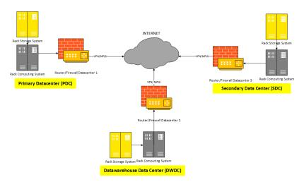
The integrated datacenter network has to provide interoperability in the Communication layer for the ANAF Common Application Architecture, described in the diagram below:
