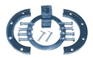
The B-84-B Break Repair Kit makes it a quick and simple job to repair a hydrant that has been damaged by traffic. This kit contains all the parts needed to replace those parts designed to break away upon impact from a vehicle.
