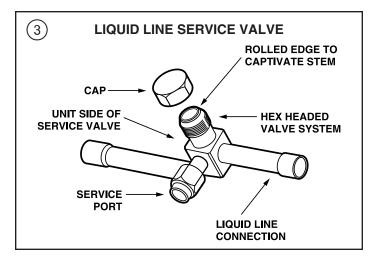
Pressure taps are provided on the service valves of outdoor unit for compressor suction and liquid pressures.
