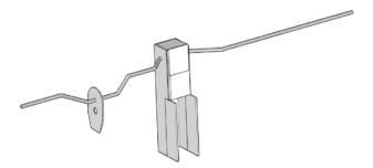
Do the same procedure with the CA glue on each of the holes in the column. Insert the Crankshaft through the holes in the column.
