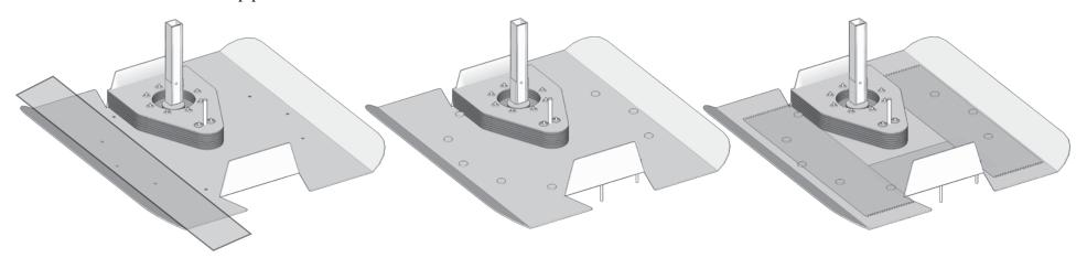
Now turn over the top plate, being careful not to squash the connecting rod. Find a large mug or small bowl and flip the Top Plate over so the rivet points are facing upwards and the stack of cardboard around the diaphragm is inside the mug. Remove the protective covering from the plastic strip and bend the strip into a circle inside the rivets.
