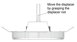
If you can't find an orientation where the displacer moves freely, turn the assembly over and mark with a pen on the bottom of the displacer where it contacts the side of the cylinder. Remove the displacer and **gently** sand the marked side. Repeat these steps until you have a displacer that moves freely up and down.
