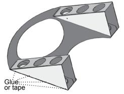
To assemble the flywheel, put one of the large disks smooth side down and place 8 small drops of glue (or double-stick tape) around the edge of the disk, and then stack the other large disk smooth side up on top, using the holes to align the two. A book can be carefully placed on top to hold them flat while they dry.
