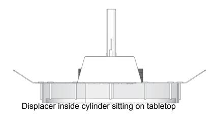
Once the epoxy has cured, try lifting the displacer rod and releasing it to make sure that the displacer moves freely. If the displacer binds, try rotating the displacer by twisting the rod slightly and repeat the lifting and releasing.
