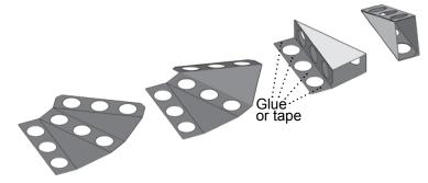
When both parts are dry, glue (or use double-stick tape) to mount the smaller piece onto the larger one as in the drawing to the right.
